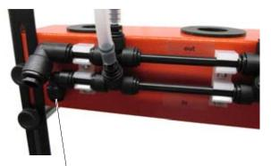
Push the supply hose firmly into the socket on the lower distributor line as far as it will go
